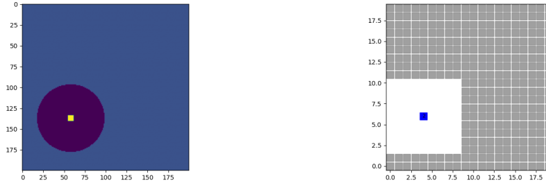
Figure 8: Range for DME-DRL Robot Sensor (left), compared with range for Benchmark Robot Sensor (right). Note that blue (left) and gray (right) cells represent unknown cells, while purple (left) and white (right) cells represent free space. The yellow square on the left is the robot and the blue square on the right is the robot.
